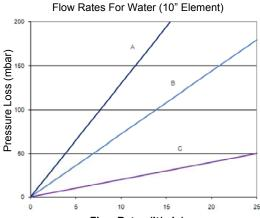
Flow Rates (It/min) A=0.03μm B=0.1μm C=0.2μm
