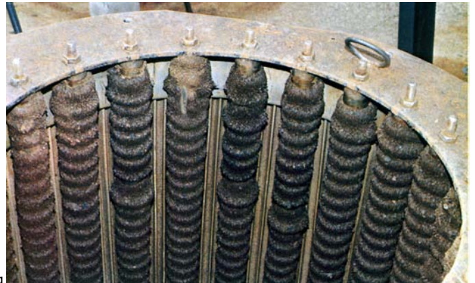
Loading inside the filter
