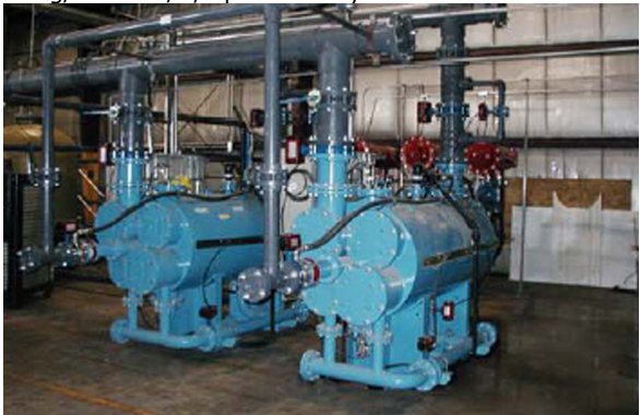
Vegetable canning operation. 170 m 3 /h, 3μ. Wisconsin, USA
