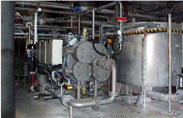
Paper mill manufacturer. Reduce TSS from 12 mg/l to 3 mg/l. 40 m 3 /h, 3μ. Germany
