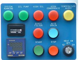
**Operator Friendly Smart Relay -** Smart relay enabled control panel performs controlled start-up & shut-down routines for ease of operation and keeps operators out of the control box. Includes machine drain sequence & automatic phase reversal (internally controlled, no guess work or switch to
